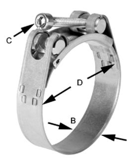
C (screw type) = ISK Diameter D = 112-121Width B = 25
